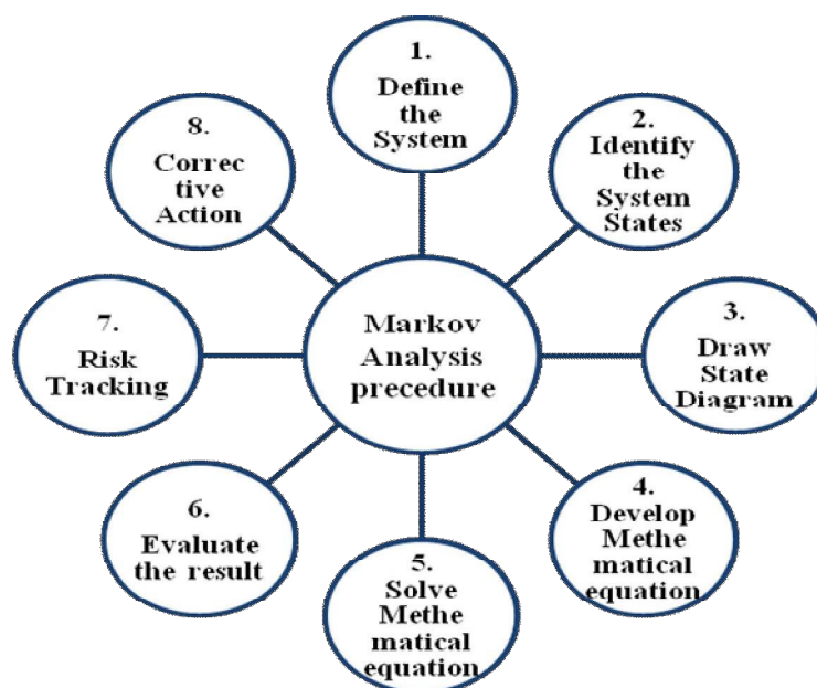
Figure 6.3 Markov Analysis Procedure
