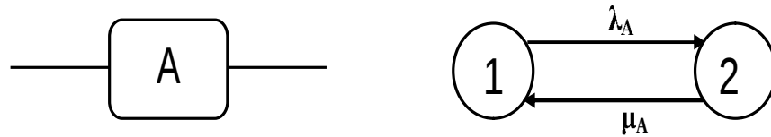
Figure 6.4 State Transition Diagrams for Single Component with of two states
